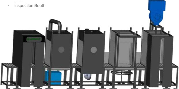
Magnaflux's modular penetrant equipment design makes it simple and cost-effective to build the right equipment for every process, including water wash, lipophilic and hydrophilic LPI testing, while also conforming easily to fit the required work flow and available floor space with straight line, U-shaped and L-shaped designs.
