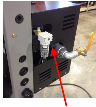
Incoming Air Connection 1/8" NPT Thread
